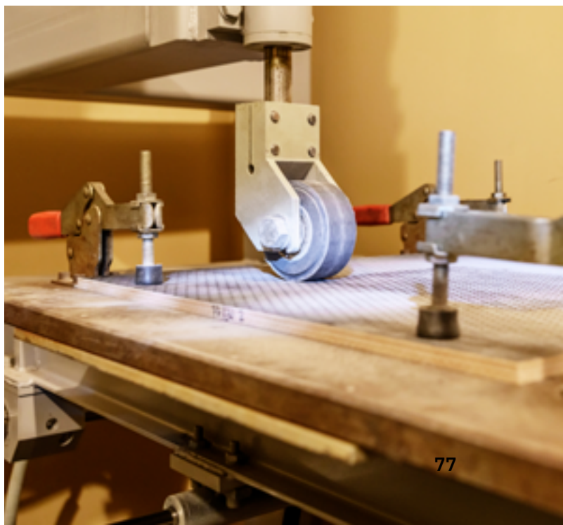
Figure 3.4. Determination of the effect of loaded heavy duty castors
